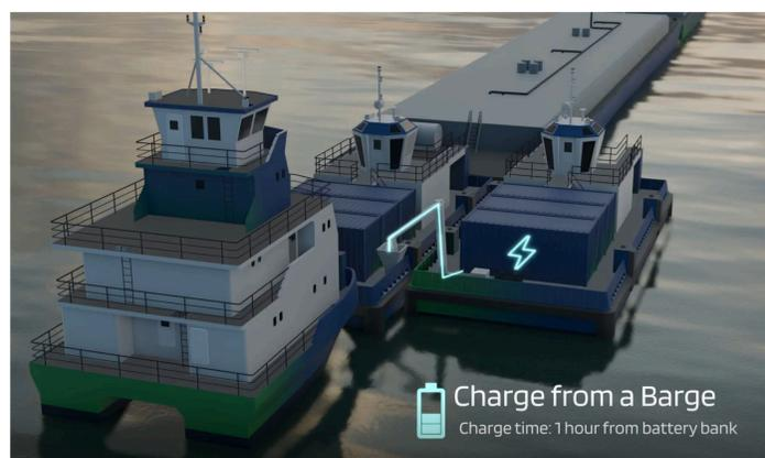
Charging of battery containers can occur from the dock, from the barge, or by swapping containers.
